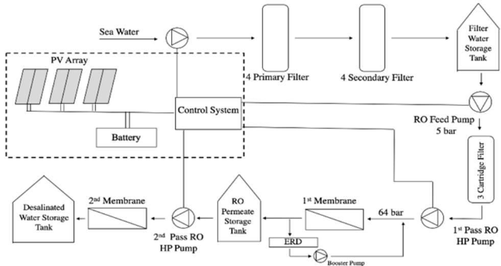
**Fig. 2. PV power supply for reverse osmosis desalination plant**
