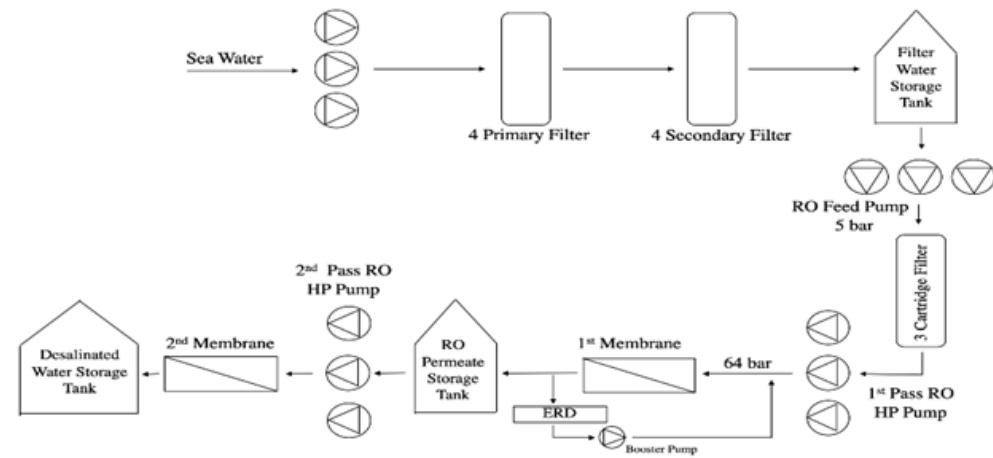
**Fig.1.Reverse Osmosis (RO) Schematic Diagram**
