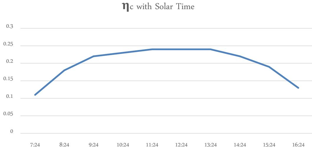
**Fig.3: Collector efficiency  $\eta_c$  with Solar Time**
