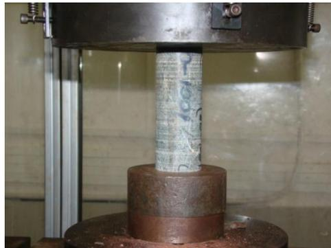
**Fig.6. A sample under UCS test**
