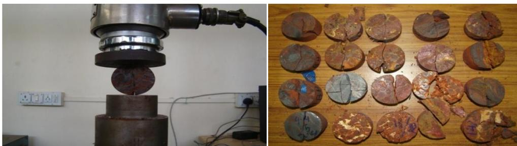
Fig. 14 Samples under Uniaxial Tensile Strength test (Brazilian test)
