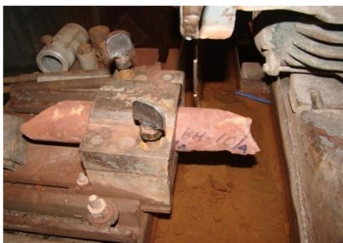
**Fig.2. Cutting by diamond circular saw**
