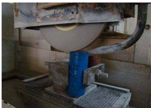
**Fig. 4. Polishing by grinding machine**
