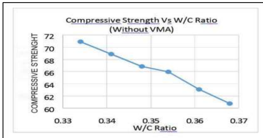
Fig.2.Variation of compressive Strength with w/c ratio without VMA addition
