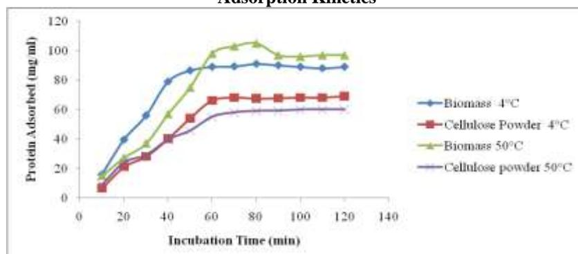
Figure 6 : Effect of incubation time on protein adsorption at different temperatures
