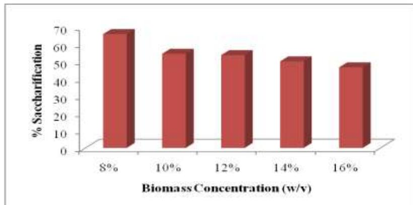
Figure 2: Optimization of solid to liquid ratio for acid treated sorghum biomass
