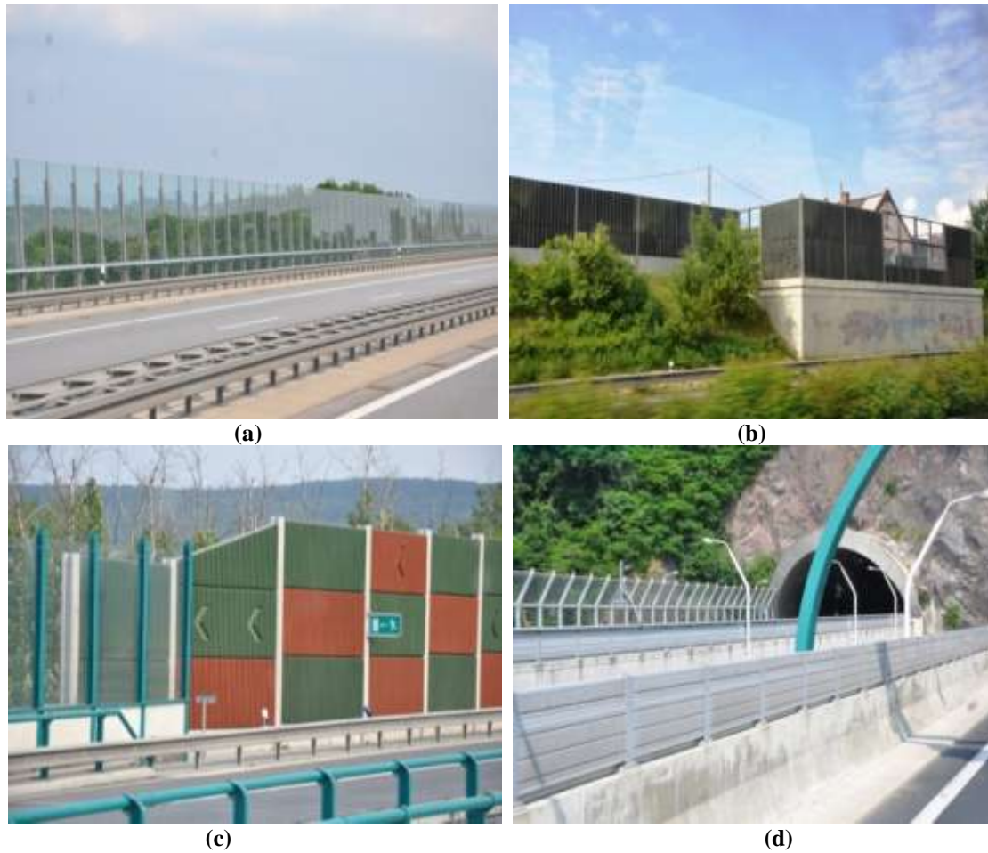
Figure 4. (a) Transparent noise barrier, (b) Metal noise barrier, (c) Concrete noise barrier, (d) Plastic, PVC and fiberglass noise barriers
