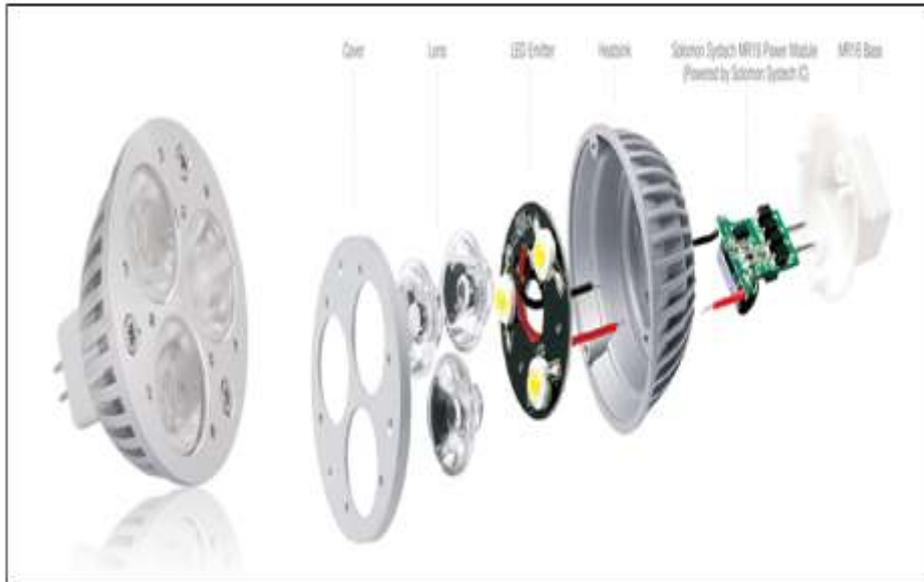
Fig.1. Exploded view of MR16 3W LED
