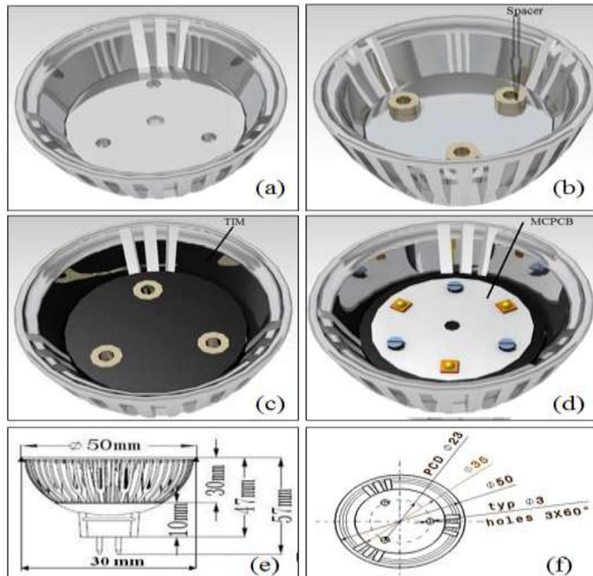
Fig.3.Sequence of assembly of LED lighting load with TIM (a) Heat Sink (b) Spacers in place(c) TIM spread (d) MCPCB placed above TIM; (e) and (f) Dimensioned views of the Lighting.
