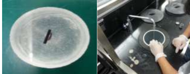
Figure 6: (a) specimen for SEM imaging (b) polishing of specimen to expose surface of interest in SEM
