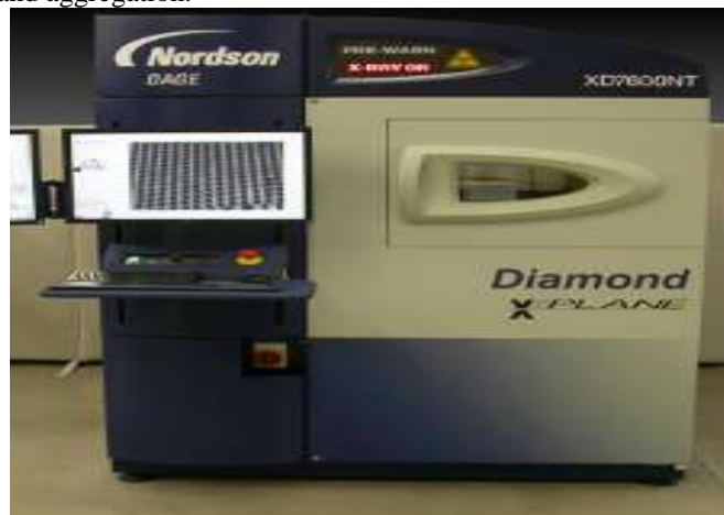
Figure 5: X-ray machine to observe outgassing paths of sinter Ag die attach materials
