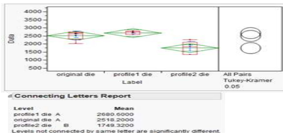
Figure 10: Tukey-Kramer Plot for statistical significance for Original, Profile 1 and Profile 2.
