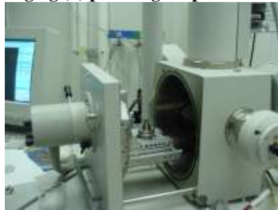
Figure 7: SEM equipment to analyze the morphology and degree of agglomeration and aggregation among sinter paste
