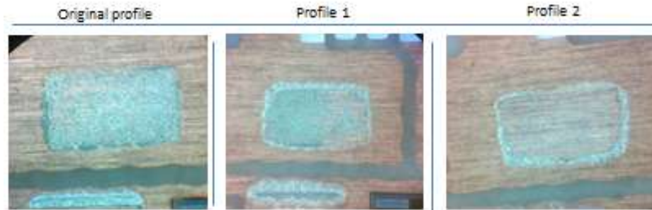
Figure 12: Optical Inspection of lead frame and sheared die indicating Less remnants of sinter Ag pastes at profile 2.
