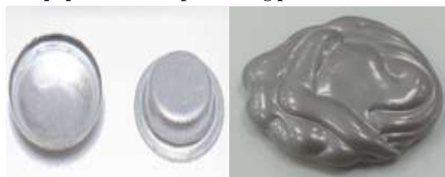
Figure 3: Aluminum Pads used for TGA; Figure 4: Sintered Ag die attach material
