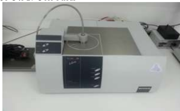
Figure 2: TGA equipment for the pre heating profiles of the die attach material
