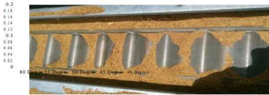
Figure 2 Corrugated types heat exchanger
