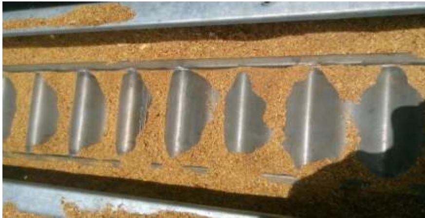
Figure 2 Corrugated types heat exchanger
