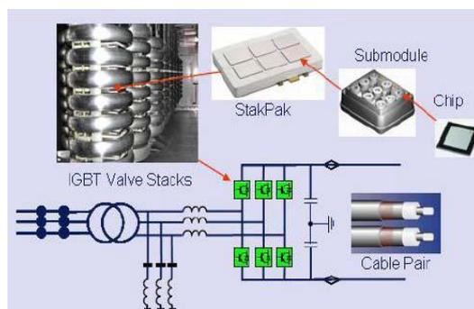
**Fig. 5. HVDC Light IGBT arrangements [4].**
