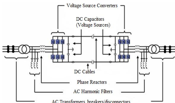
**Fig. 4. Simplified circuit diagram for 2-level VSC-HVDC showing the major components of the system [3]**
