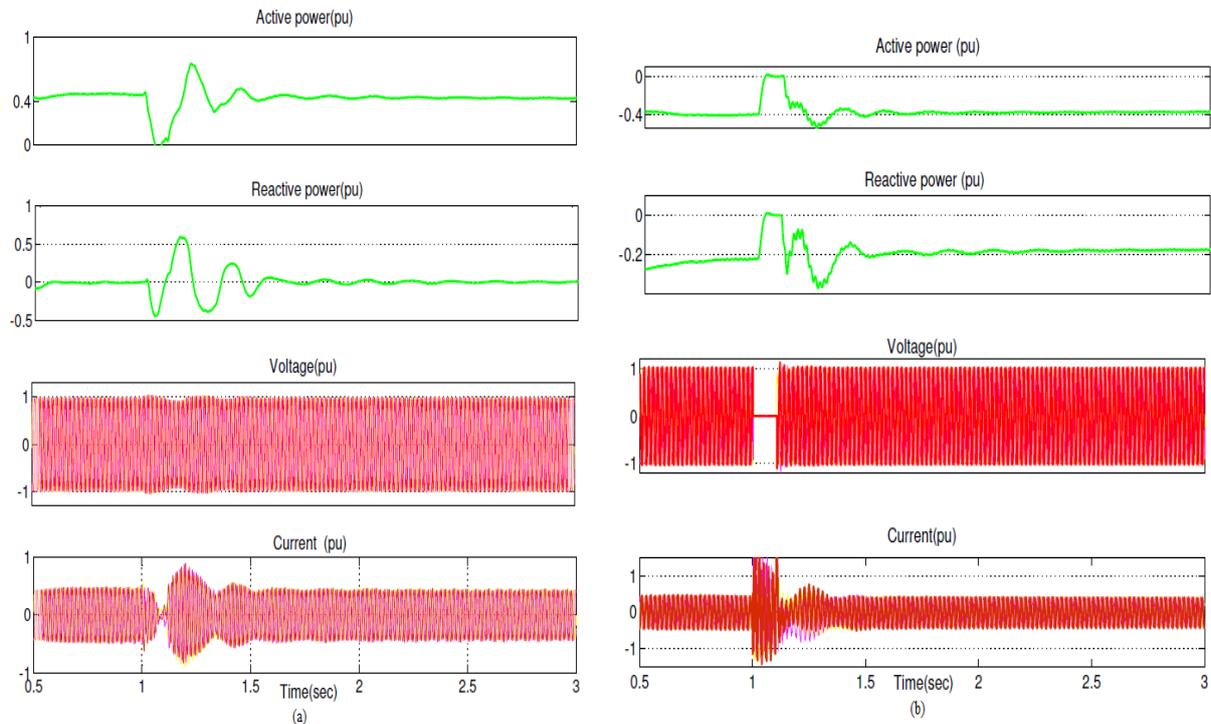
**Fig. 12. Three phase fault waveforms for HVDC Light system for fault at  $t=1.0s$  at station 2 side end, (a) Station 1 side (Rectifier) (b) Station 2 side (Inverter).**
