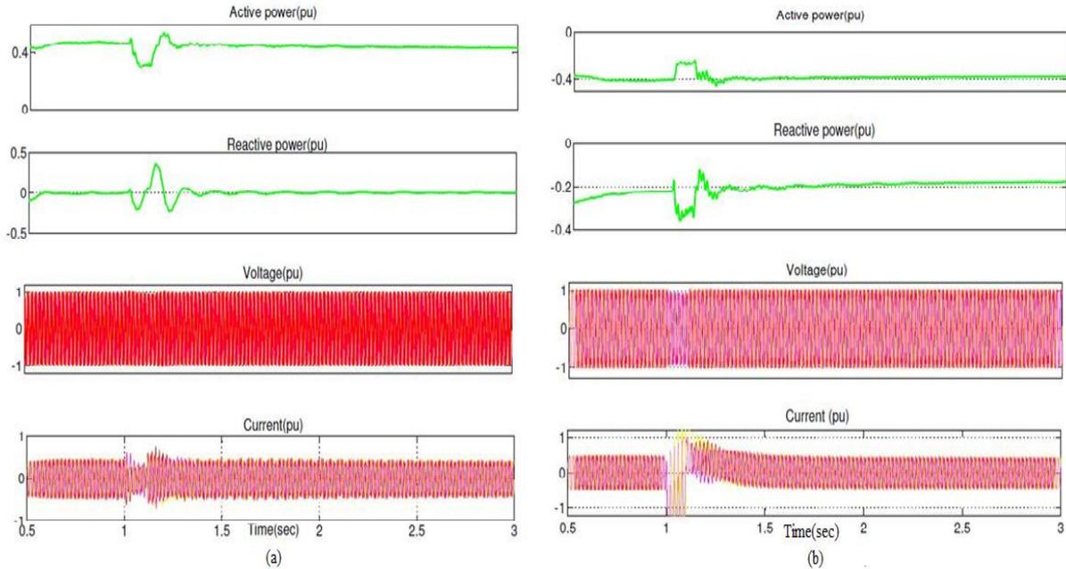
**Fig. 11 Single phase to ground waveforms for HVDC Light system for fault at  $t=1.0s$  at station 2 side end, (a) Station 1 side (Rectifier) (b) Station 2 side (Inverter)**
