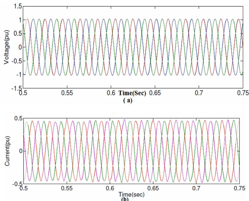
**Fig. 10 Simulation results of the voltage and current when the HVDC Light system is under steady state operation condition.**
