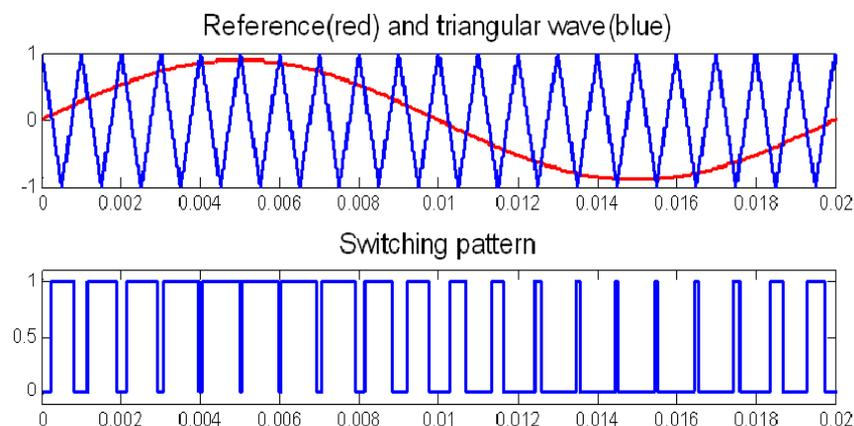
Fig. 2 Reference and Carrier Waveforms Compared to form PWM Switching Pattern
