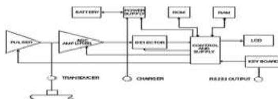
Fig. 3.6 block diagram of a modern microprocessor-controlled ultrasonic gauge
