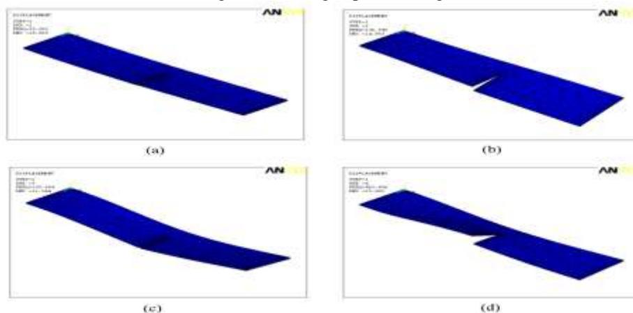
**Fig. 5.5** a) 1<sup>st</sup> Bending mode at 38.08 Hz b) 1<sup>st</sup> Torsion at 136.55 Hz
