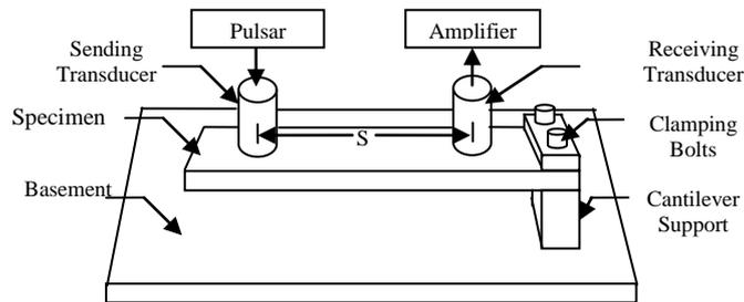
Fig. 3.4 Schematic representation of experimental setup
