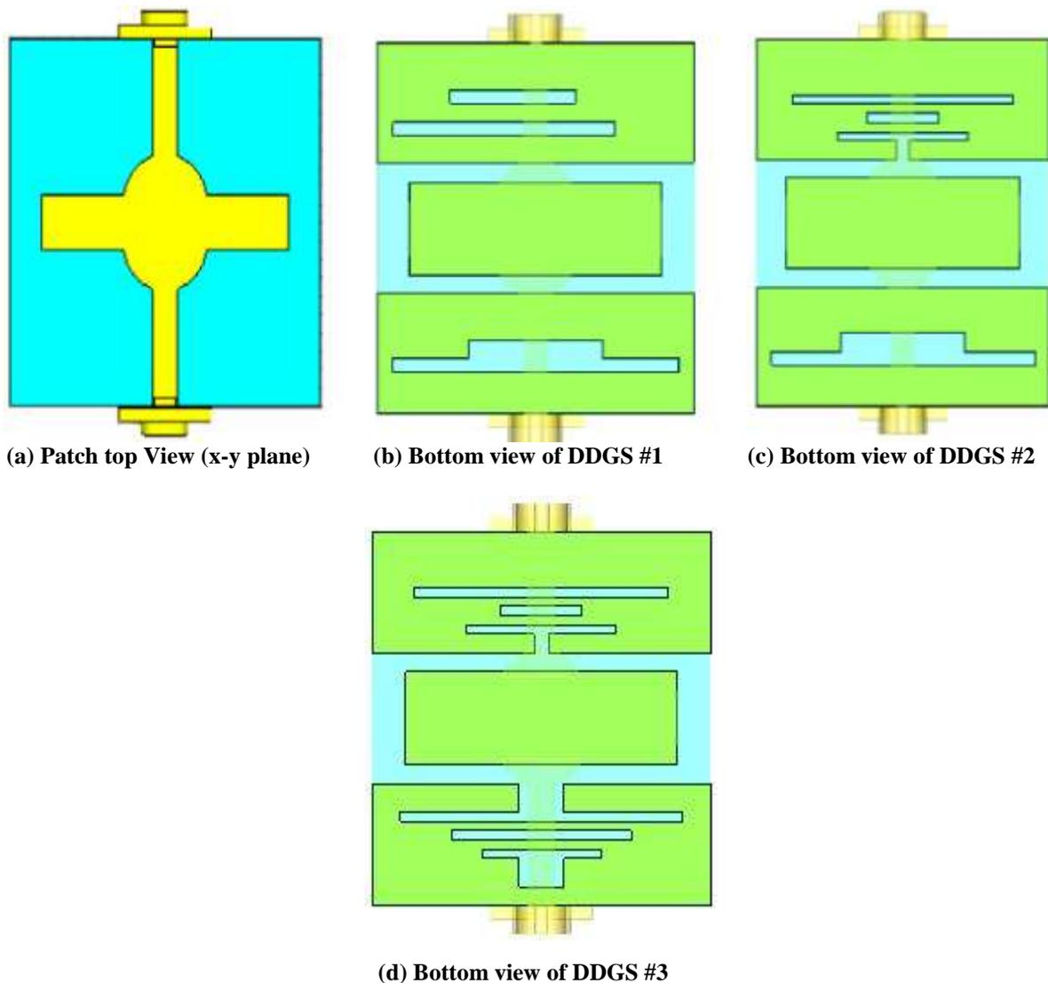
Fig.1 Proposed Two-Port microstrip antenna configuration
