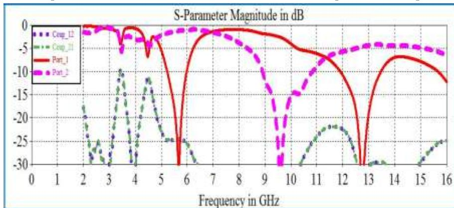
(a) S-parameters of the proposed antenna with the first ground configuration (DDGS #1)
