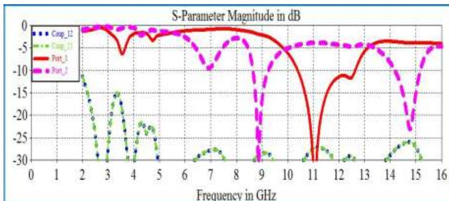
(c) S-parameters of the proposed antenna with the third ground configuration (DDGS
