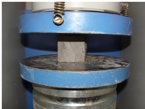
Fig. 6. Testing of compressive strength of cube
