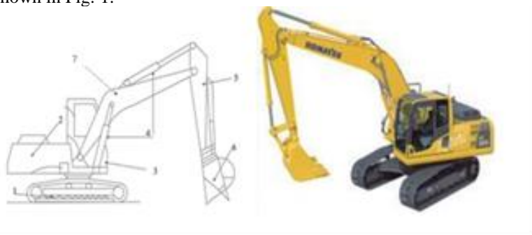
Fig. 1. 1. Undercarriage with drive system, 2. Upper structure with cabin, 3. Cabin, 4. Hydraulic cylinders, 5. Arm, 6. Bucket, 7. Boom.
