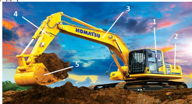
Fig. 5. 1. Cabin, 2. Engine, 3. Boom, 4. Stick, 5. Bucket
