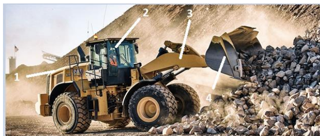
Fig. 10. 1. Engine, 2. Cabin, 3. Two-part boom, 4. Bucket
