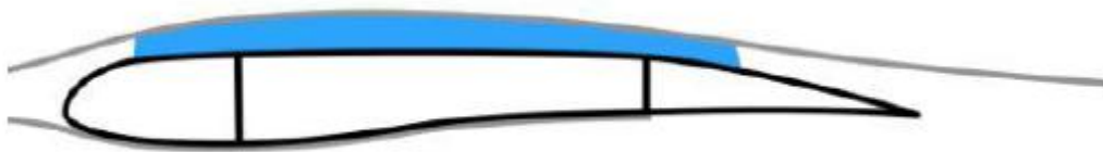
FIGURE 2 Shows the NACA 6-series airfoil with boundary layer formation on top.
