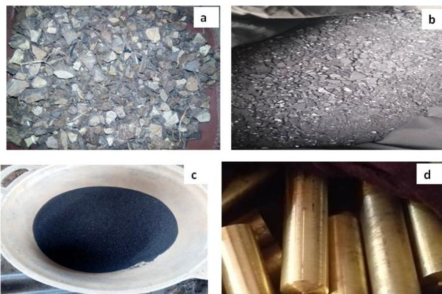
**Figure 1: (a) Coconut shell (b) Carbonized and crushed CSA (c) Sieved CSAp (d) Scrap brass**
