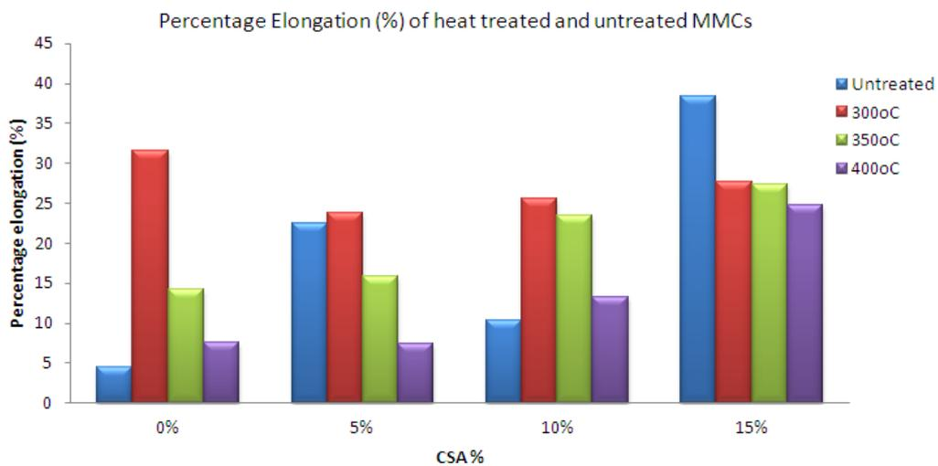
Figure 9: Comparison of percentage elongation of MMCs at varied heat treatment temperatures
