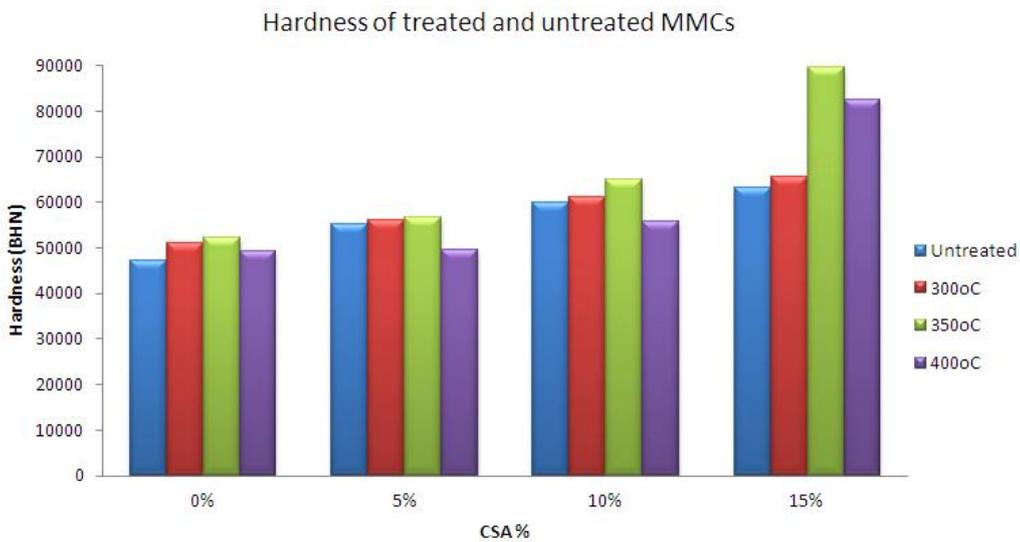
Figure 8: Comparison of hardness of MMCs at varied heat treatment temperatures
