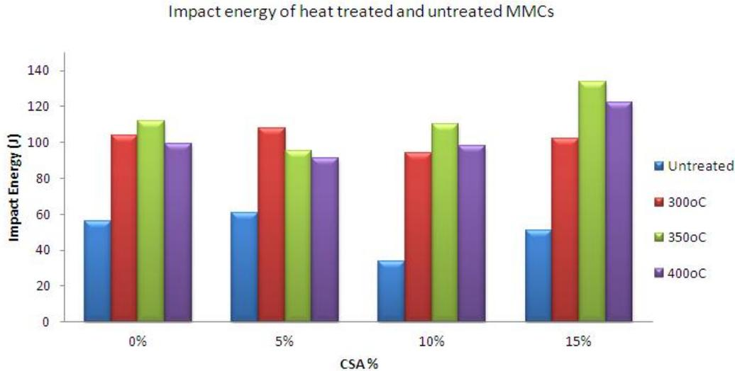
Figure 10: Comparison of impact energy of MMCs at varied heat treatment
