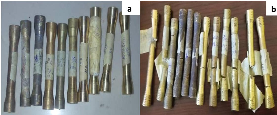
**Figure 4:** (a) Machined specimens before tensile strength test (b) Machined specimens after tensile strength test
