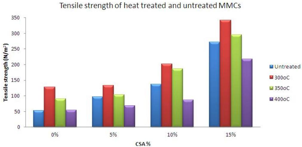
Figure 7: Comparison of tensile strength of MMCs at varied heat treatment temperatures
