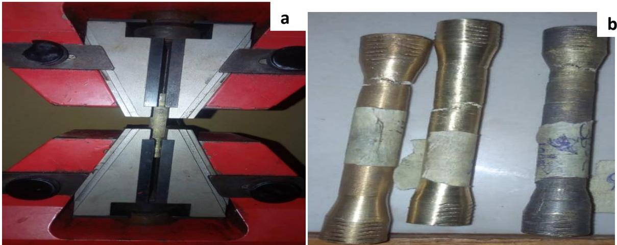
**Figure 5:** (a) Tensile strength test of the specimen using Tensile Test (circular comp)
