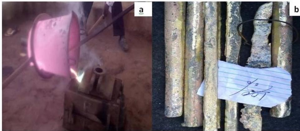
Figure 2: (a) Casting process (b) Casting products
