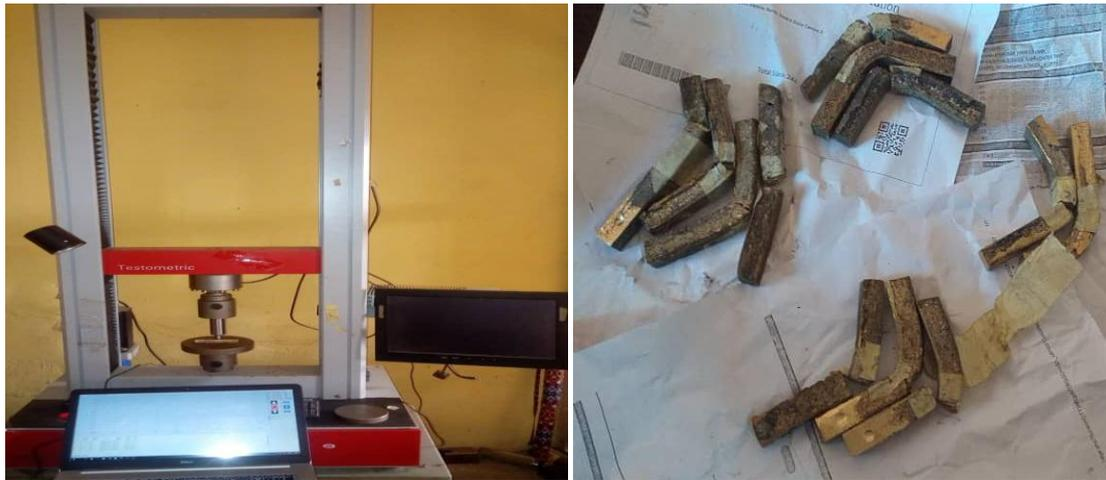
Figure 6: (a) Hardness test of the specimens using Brinell Hardness Testing machine (b) MMCs specimen after hardness test
