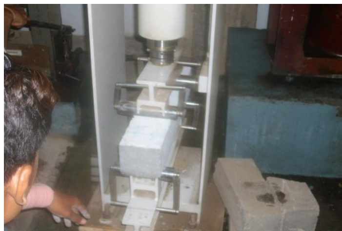
Fig. 2 “Testing of flexural strength test specimen”
