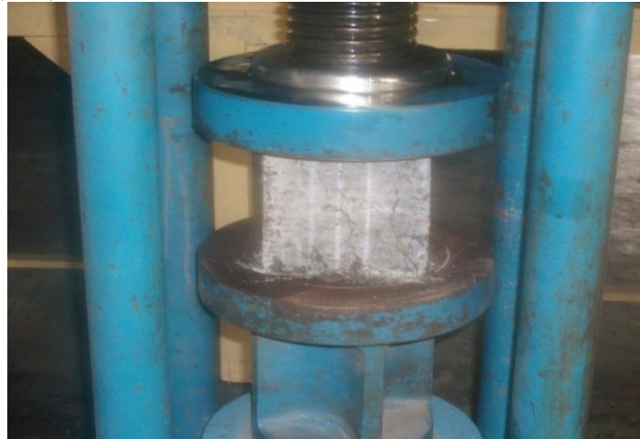
Fig. 1 “Testing of compressive strength test specimen”
