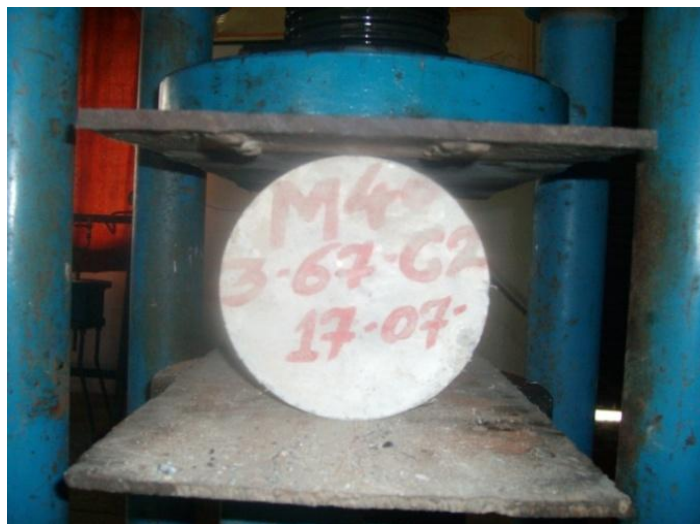
Fig. 3 “Testing of Split tensile strength test specimen”
