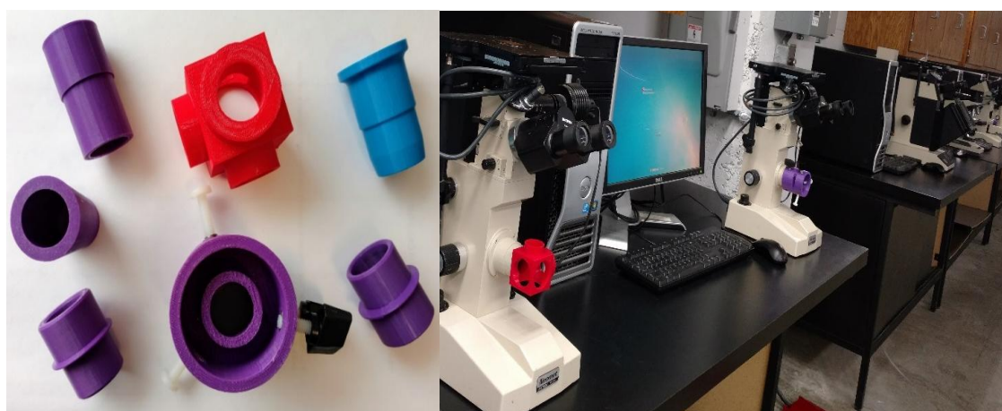
Figure 2. Various microscope-to-digital camera adaptors made of PLA
