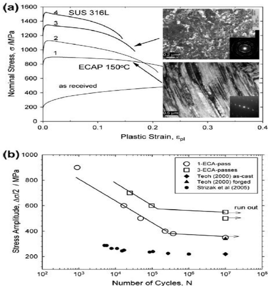
Fig 5. (a) Tensile stress–strain curves and (b) S–N fatigue plot for SUS 316L austenitic stainless steel after ECAP [147]
