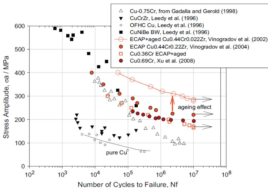
**Fig. 6** The Wohler plot comparing fatigue lives and endurance limits for conventional and SPD-manufactured Cu-based alloys (Cu–Cr and Cu–Cr–Zr)
