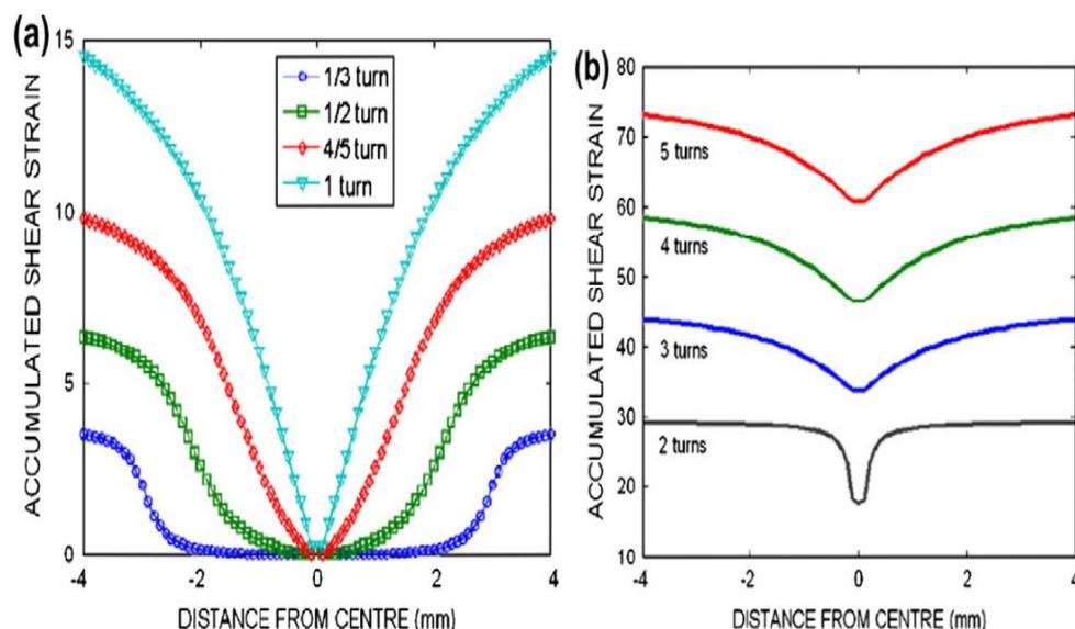
**Fig. 2.** Accumulated shear strain as a function of the distance from the torsion axis for the first-order gradient model [53].
