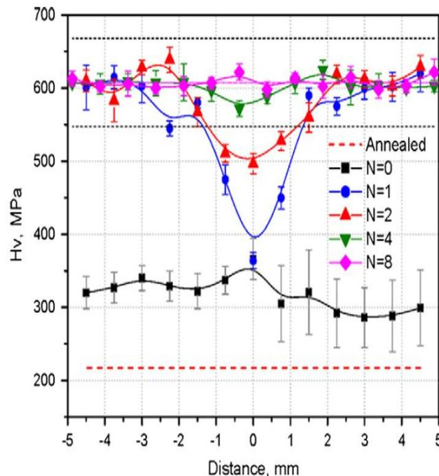
**Fig. 1** Vickers microhardness (Hv) of HPT samples after different numbers of turns (N) as a function of the distance from the centre of the specimen [53].
