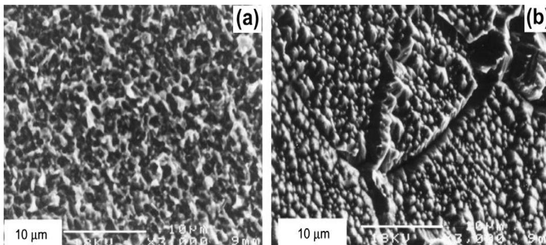
**Fig. 13.** SEM micrographs of ECAP copper (a) UFG state after ECAP and (b) a coarse-grained state after annealing at 823 K for 30 min [182].
