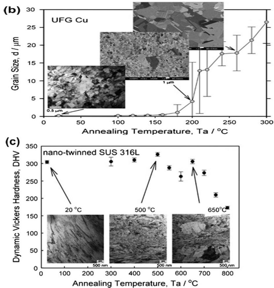
**Fig. 11** (a) and (b) Thermal stability of ECAP processed copper (99.96%), (c) SUS 316L stainless steel
