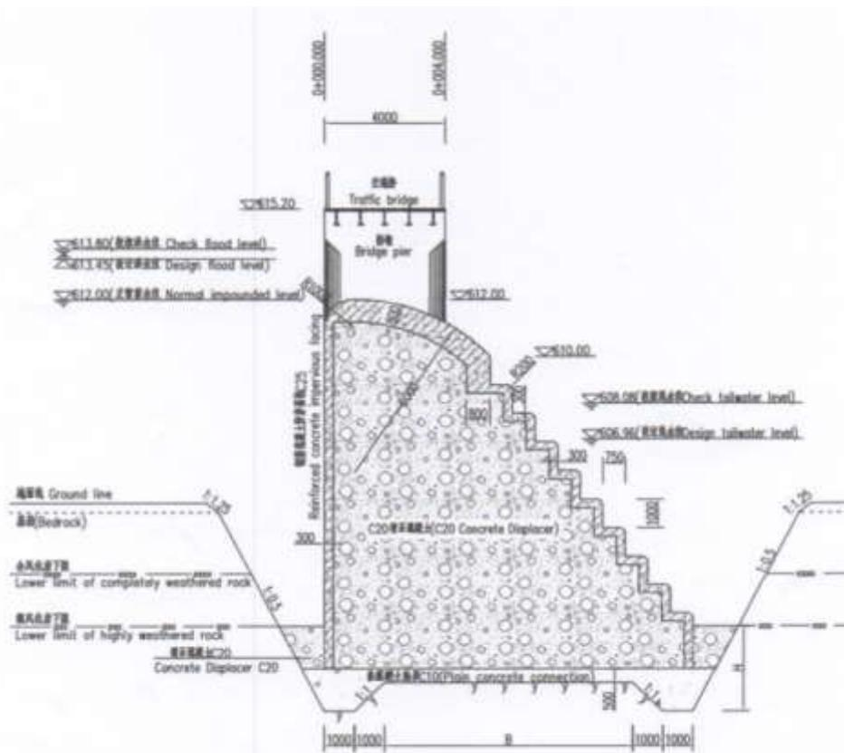
Fig. 1: Typical calculation section of overflow dam body
