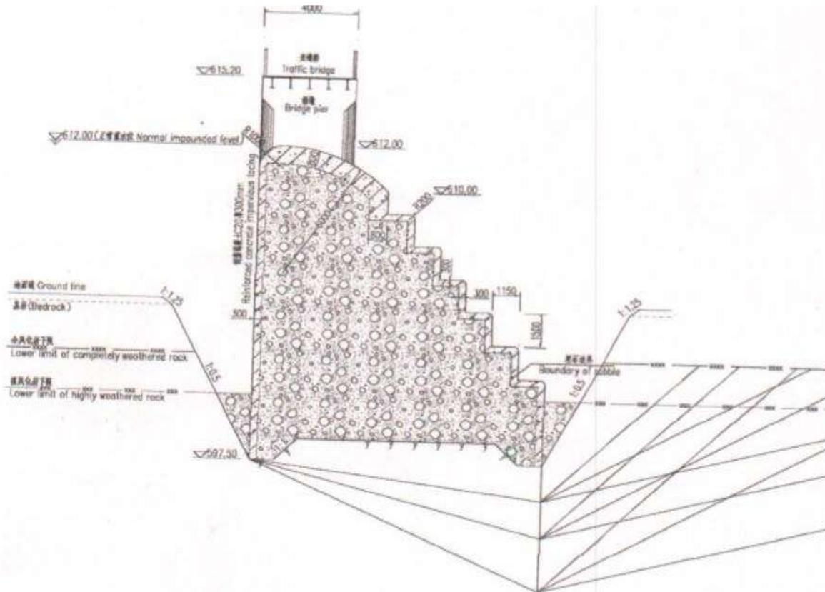
Fig. 2: Typical section for deep sliding stability of overflow dam
