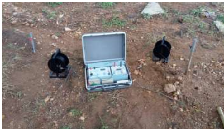
Fig.2 Arrangement for resistivity analysis
