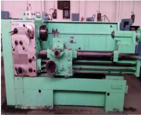
Fig.2 HMT power lathe for carrying out burnishing process.
