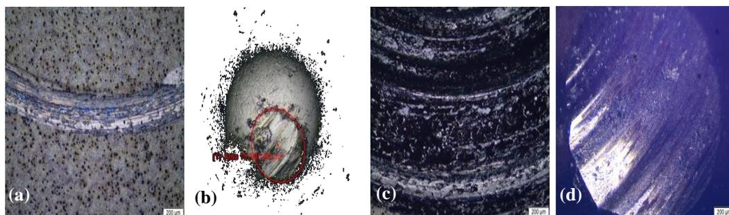
**Figure 7.** The worn surfaces under austempered conditions; applied load 10N a) the sample, b) ball bearing; applied load 30N c) the sample, d) ball bearing
