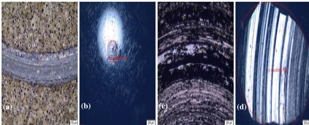
**Figure 6.** The worn surfaces under as-cast condition; under a load of 10N a) sample b) ball bearing; under load of 30N c) sample, d) ball bearing
