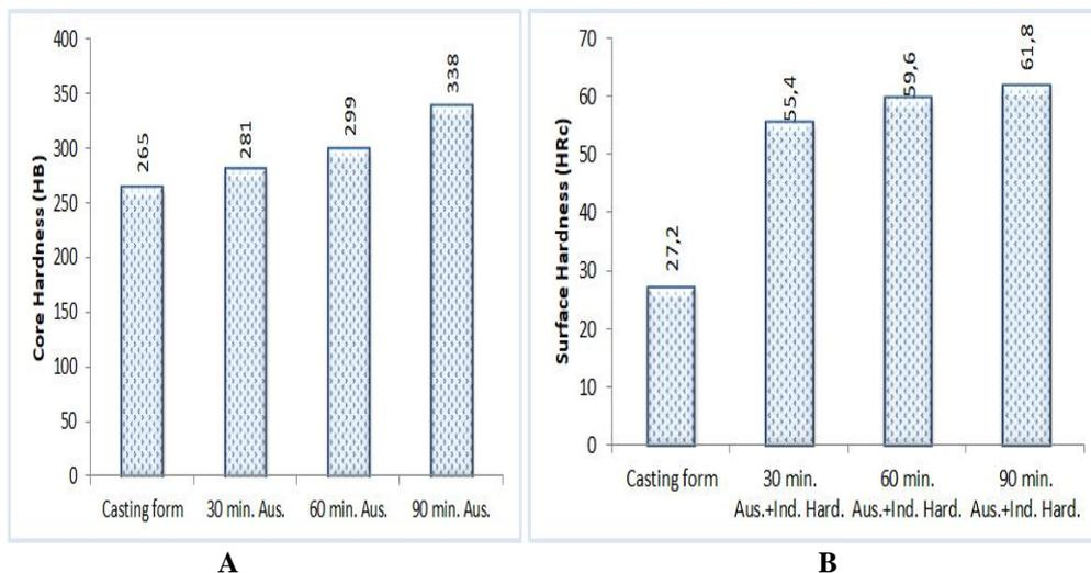
**Figure 4.** The results of hardness camshaft; a) core hardness, b) surface hardness
