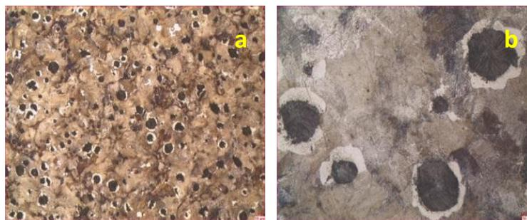
**Figure 1.** The microstructure of the cast camshaft; a) 100X, b) 500X
