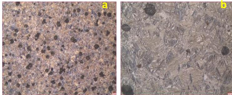
**Figure 3.** Surface microstructure of induction hardened camshaft with austempering and induction at 360°C, 90 min., a) 100X, b) 500X
