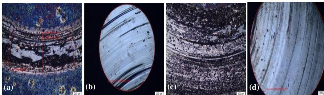
**Figure 8.** The optical microscope images of abrasion surfaces under austempered+induction hardened conditions under 10N load; a) sample b) ball bearing; 30N load c) sample, d) ball bearing
