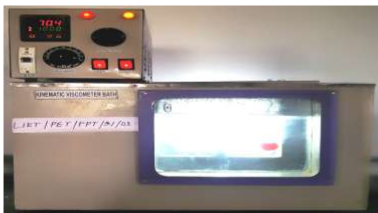
Figure 2.2: Viscometer Bath (Lab Set Up)
