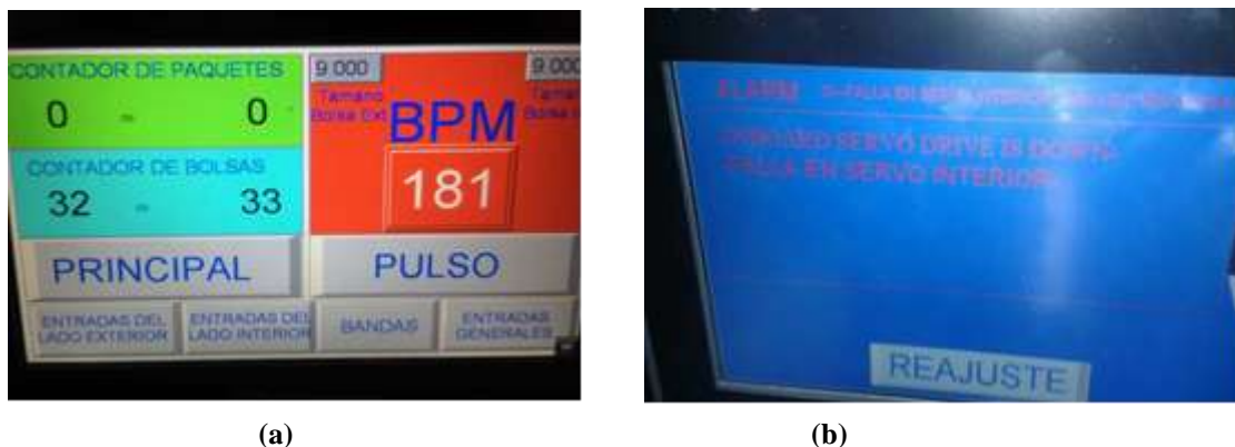
Fig. 2. (a) Control Panel of the cutter, b) failure reported "Fails in Internal Servo"
