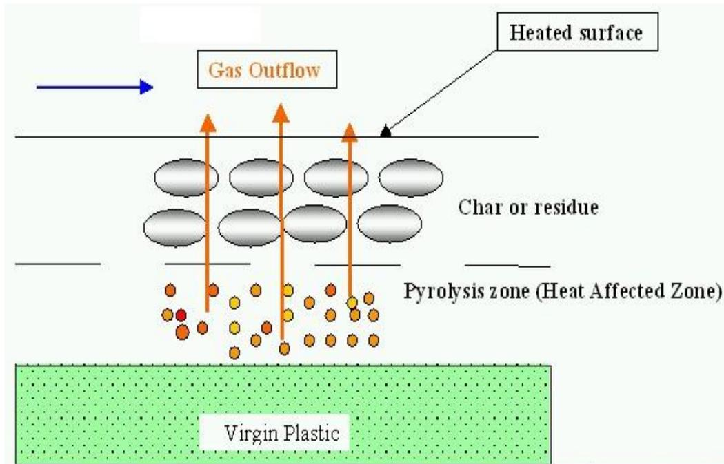
**Fig. 1: Composite degradation process**
