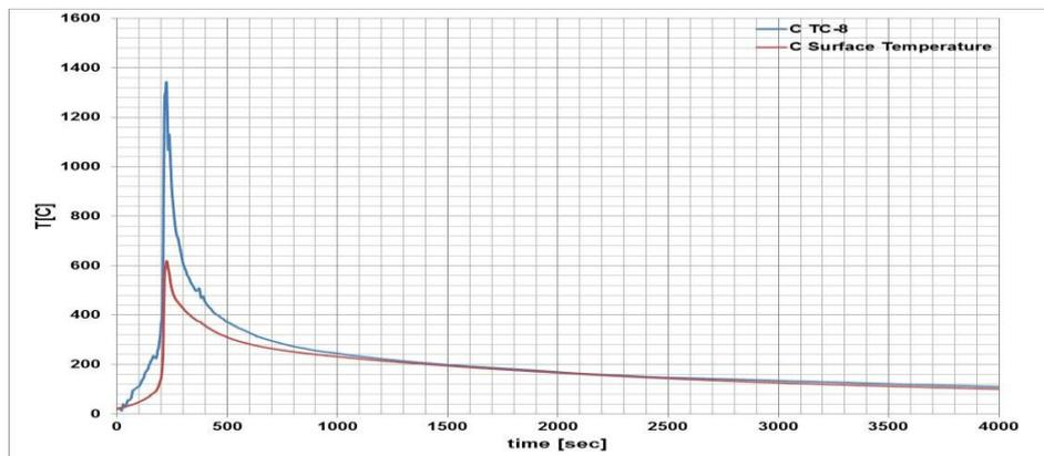
Fig. 6: Calculated thermocouple and wall surface temperatures
