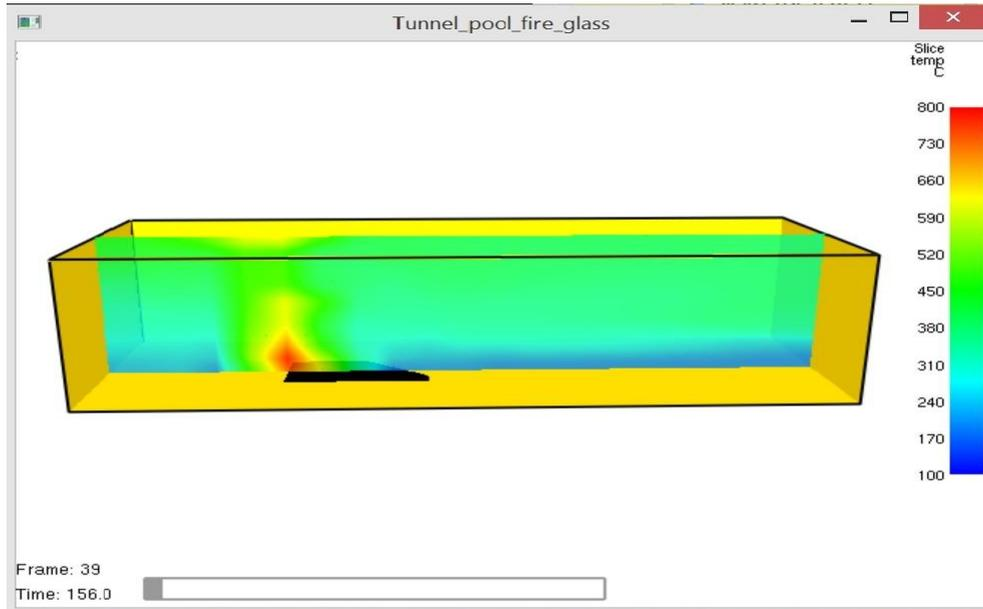
Fig. 4: Temperature field in the tunnel at t=156 sec
