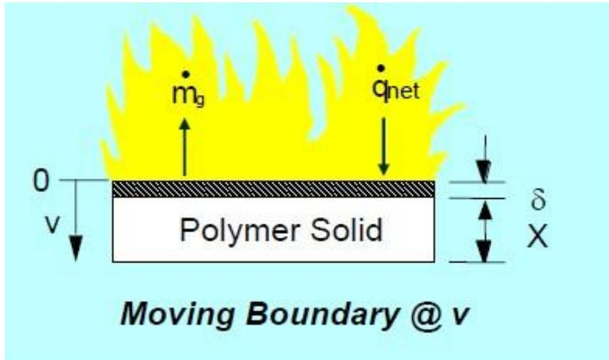
Fig 2: Burning process of polymer composite [10]
