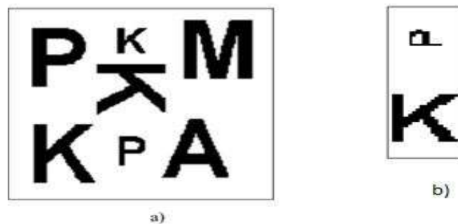
Fig .1 illustrate a pattern recognition based on the template matching approach. Fig .1.a is the input image I, Fig.1.b represents two templates (K representing letter 'K' and P letter 'P'). Input: pixels output: as correlation, distance measure function.
