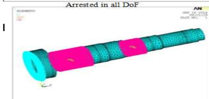
Figure 2: Bearing Locations and Face Arrested in all DoF
