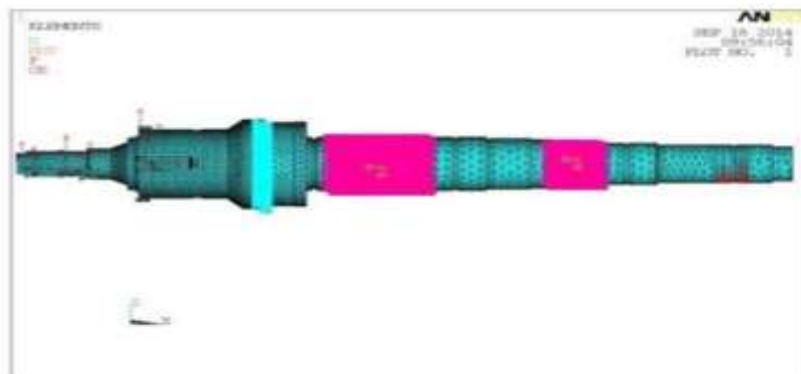
Figure 10: Belt Load Applied at the belt Location for Case 2 Analysis
