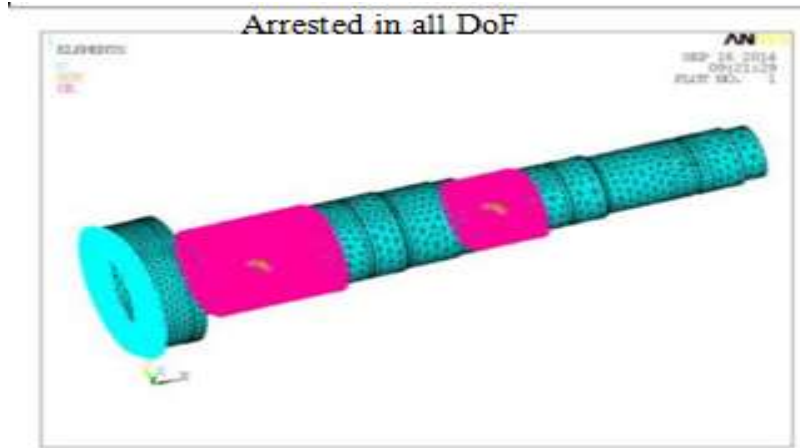
Figure 3: Belt Load Applied at the Belt Location
