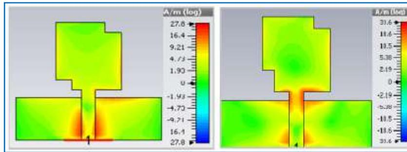
(b) Symmetric and Asymmetric edge slots for PG configuration
