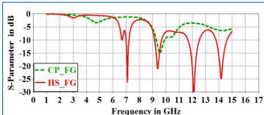
Fig.3 |S11| of H\_slot filtenna for FG configuration versus CP antenna
