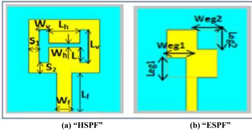
Fig.1 Top view of two proposed filtenna structures
