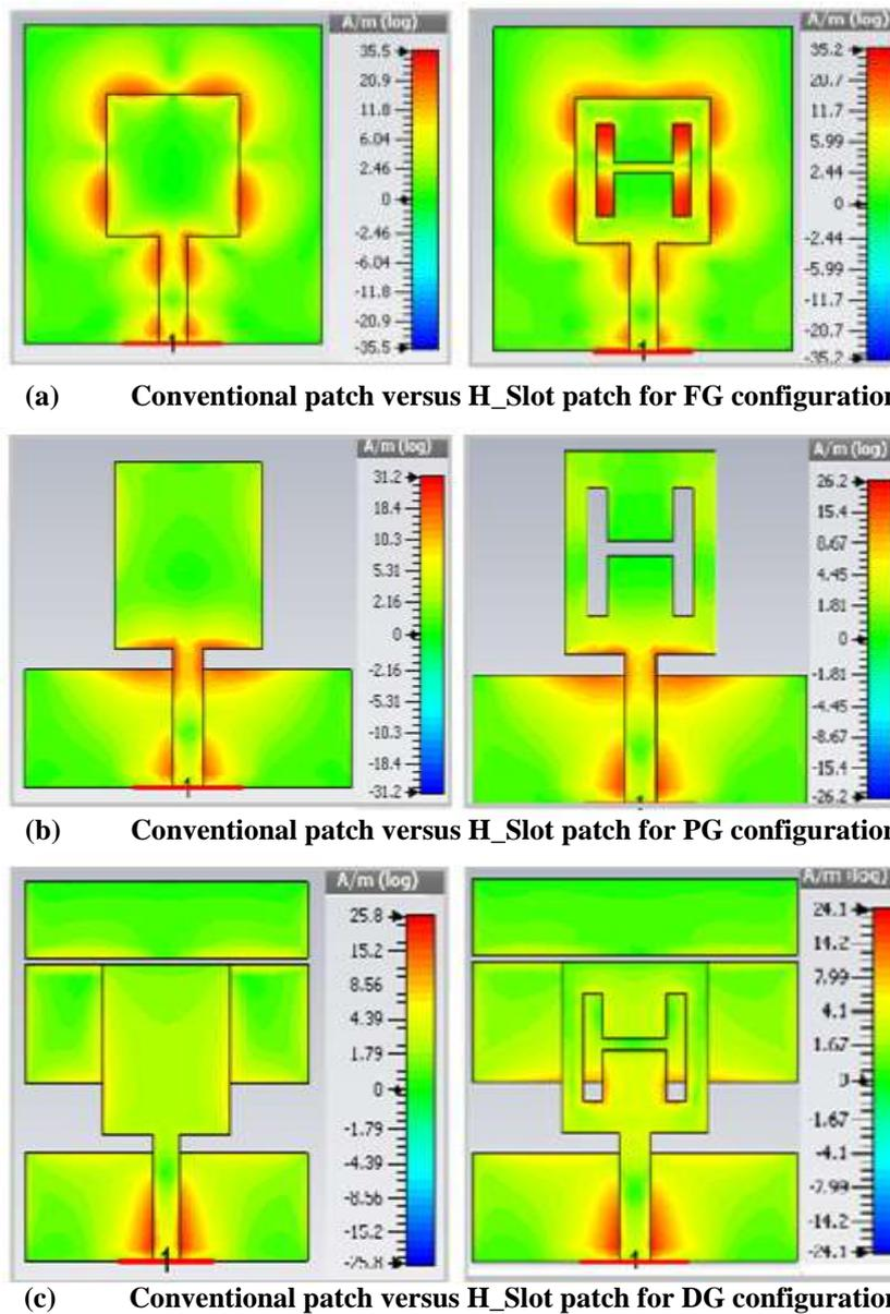
Fig.6 Current distributions of CP and HS for FG, PG and DG at the frequencies listed in TABLE 2
