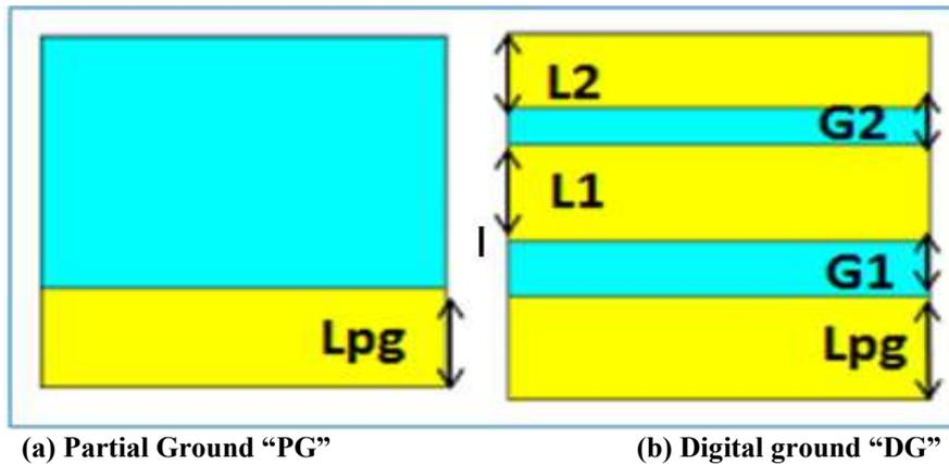
Fig.2 Bottom view of two ground configurations
