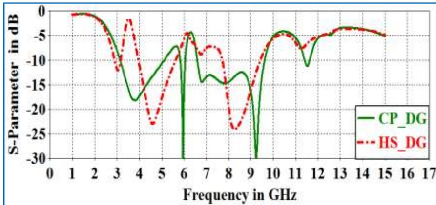
Fig.5 |S11| of H\_slot filtenna for DG configuration with ( $L_{pg}=8.5$  mm) versus CP antenna ( $L_1= 9.5$  mm,  $L_2= 6.0$  mm,  $G_1=5.5$  mm, &  $G_2=0.5$  mm)
