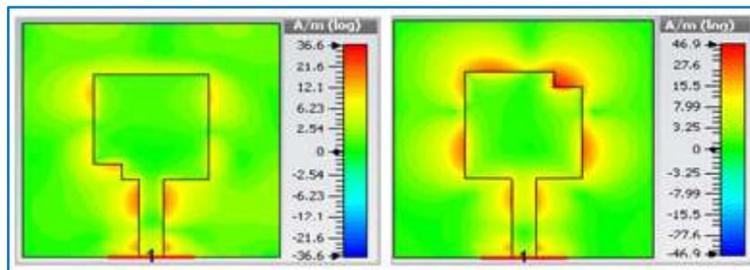
(a) Lower and Upper edge slot for FG configuration
