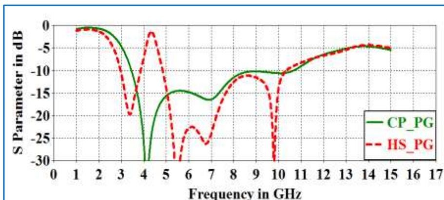
Fig.4 |S11| of H\_slot filtenna for PG configuration with ( $L_{pg}=8.5$ mm) versus CP antenna
