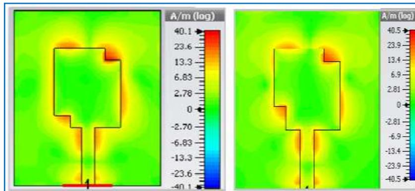
(a) Symmetric and Asymmetric edge slots for FG configuration
