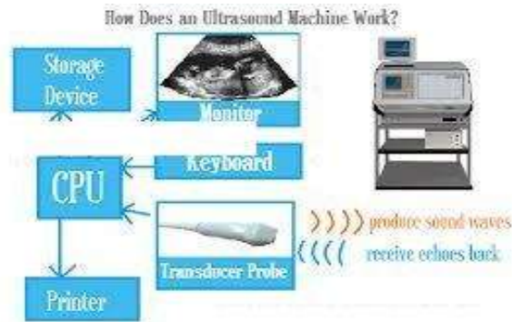
Fig 1. Major Parts of an Ultrasound Machine and Workflow
