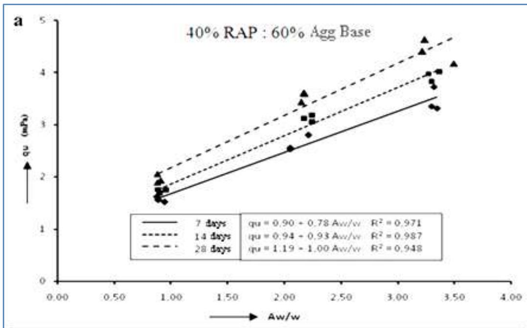
Figure 3. UCS ( $q_u$ ) Vs  $A_w/w$  ratio at 7, 14, and 28 days of curing time.
