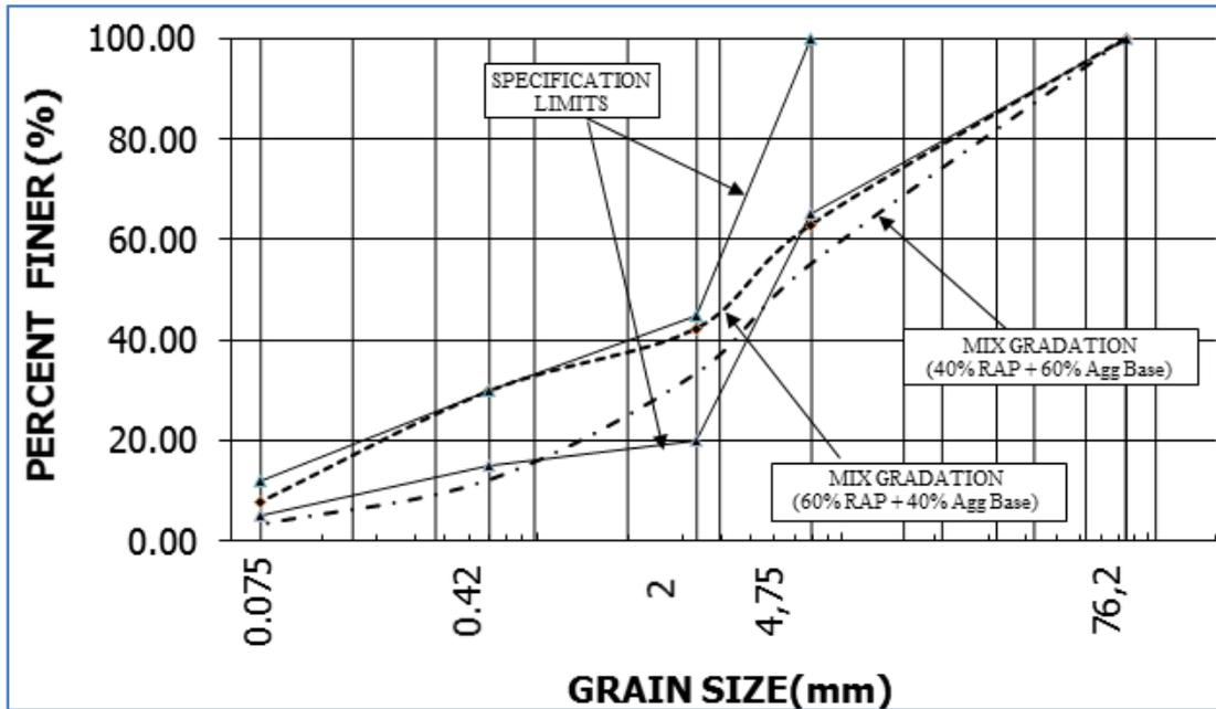
Figure 1. Grain-size Distribution of RAP and Aggregate Base Materials
