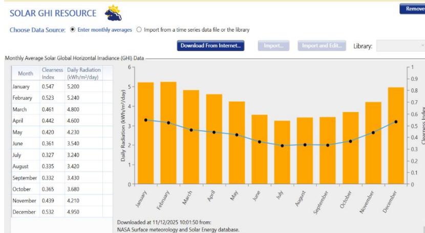
Fig3b: Monthly average solar irradiance of Igwuruta, Rivers State (kWh/m 2 /day) (src: Homer)
