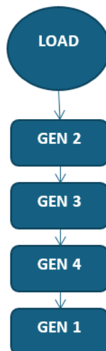
Figure 4: Order for Generator Coordination and Scheduling
